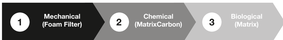
Figure 5: Layering Filtration Media (bottom to top)
